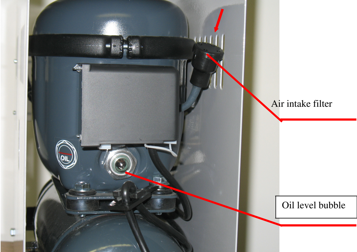
Fig.3 Rear of the compressor
