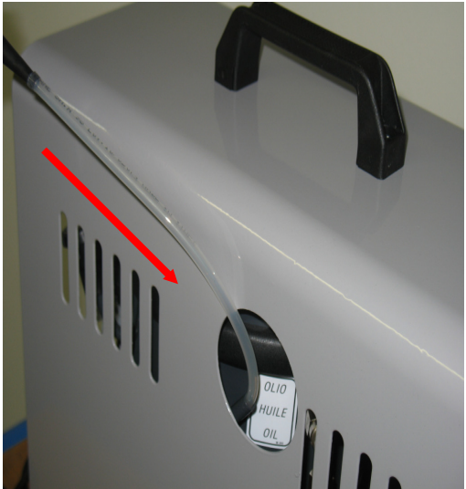
Fig.4 Oil filling from side of the compressor
