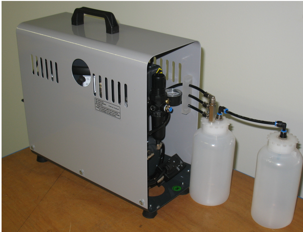
Fig. 1 Compressor with “Double drain bottle system.”
